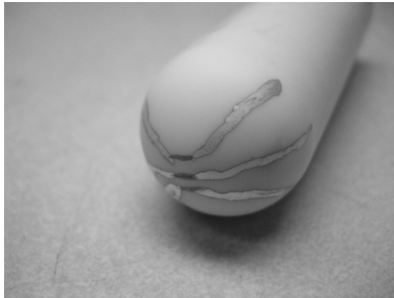
Figure 3.3: Three thin film gages painted on the stagnation region of a 25.4 mm diameter MACOR® substrate model.
