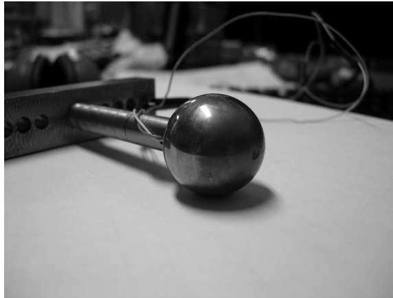
Figure 3.1: Thermocouple mounted at the stagnation region of a 25.4 mm diameter sphere model.
