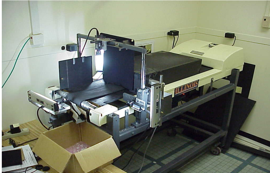
Figure 2.12 Photo of the University of Illinois Aggregate Image Analyzer (UIAIA)
