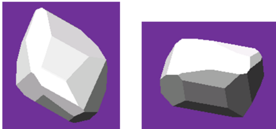
Figure 3.5 Two Views of the Generated BLOKS3D Element Based on the Desired Particle Shape Indices
