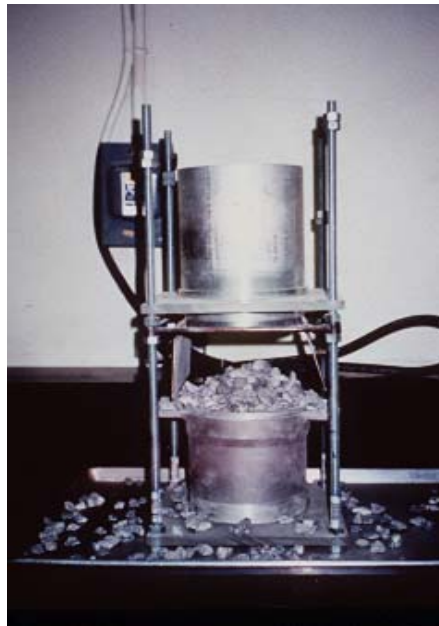
Figure 2.16 Test Setup for Uncompact Voids in Coarse Aggregate (AASHTO
