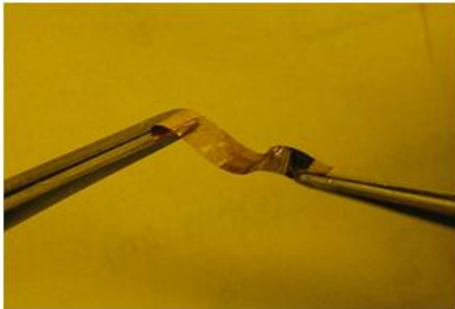
Figure 4.1 Demonstration of the mechanical flexibility of the CNT strain sensor.
