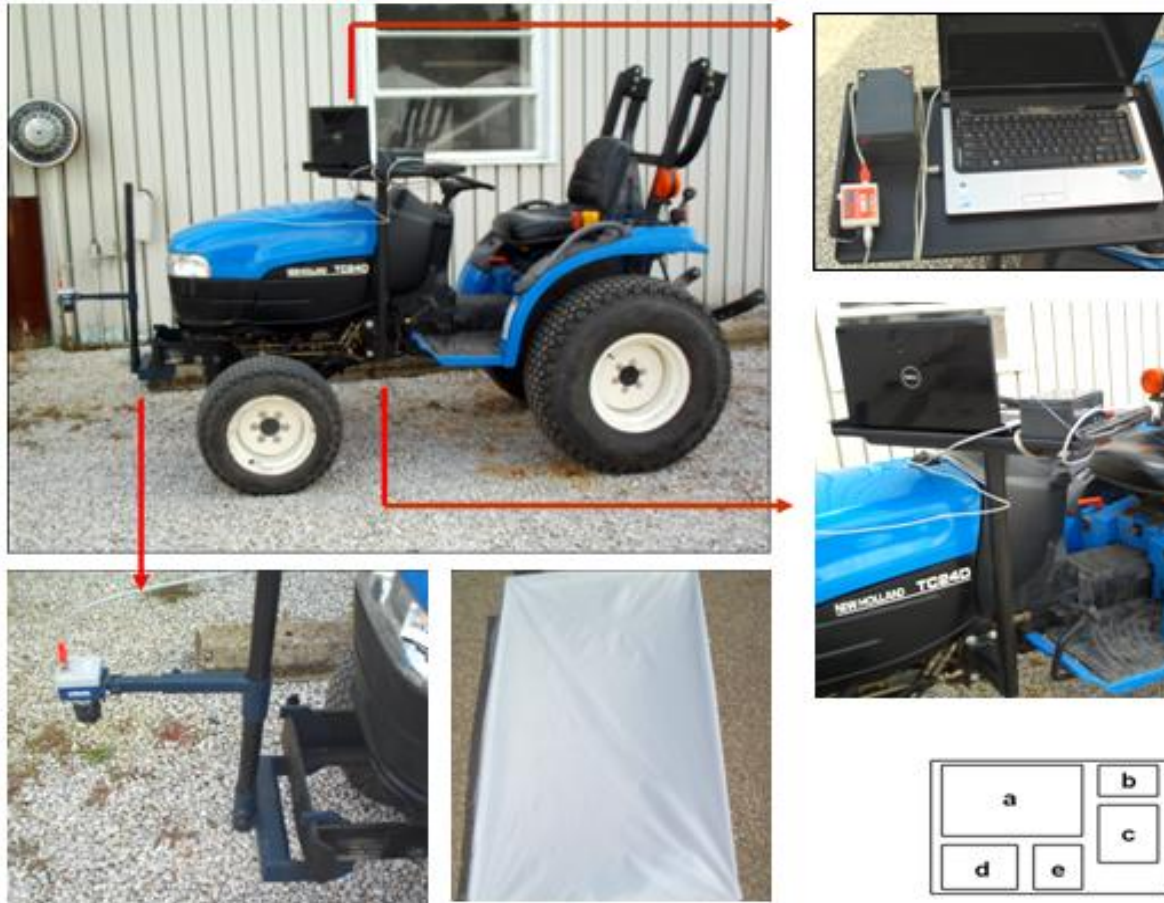
Figure 3.12. Facilities used for image acquisition during the field test.
