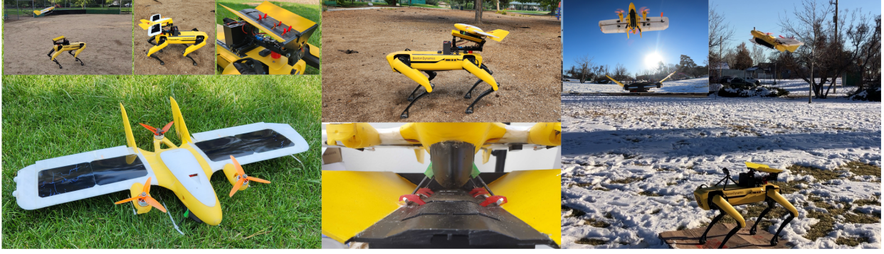
Fig. 2 Indicative illustration of our team’s autonomous self-sustainable UAVs with solar and external-battery-powered recharging capabilities, and legged-locomotion UGVs that carry Docking-&-Recharging backpacks, allowing for their combined marsupial operation as Systems-of-Systems that can support wide-area deployments in-the-wild. Such classes of systems comprise the main paradigm considered as the target application field for this paper’s proposed framework.
