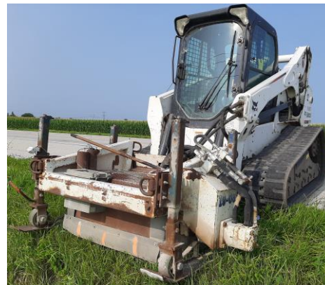
(b) Bobcat loader with asphalt planer
