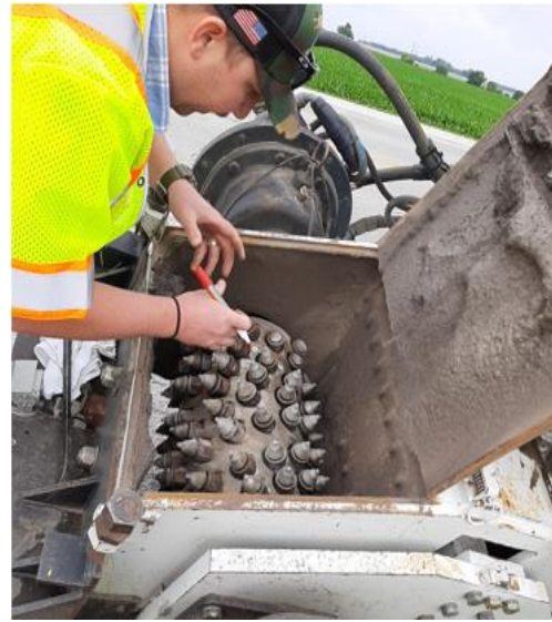
(b) Milling drum for sinusoidal rumble strip
