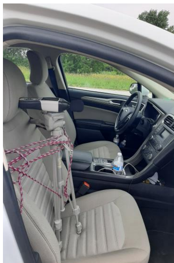
Figure 21. Photo. Equipment setup for internal noise measurement.
