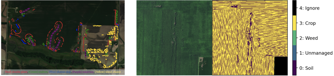
Figure 3.1: Left: Full-field imagery (RGB-only) constructed from the AV dataset. A field of this size is approximately 15,000 \times 15,000 pixels which can yield many smaller tiles. Right: Sample imagery and labels for the fine-grained segmentation task.
