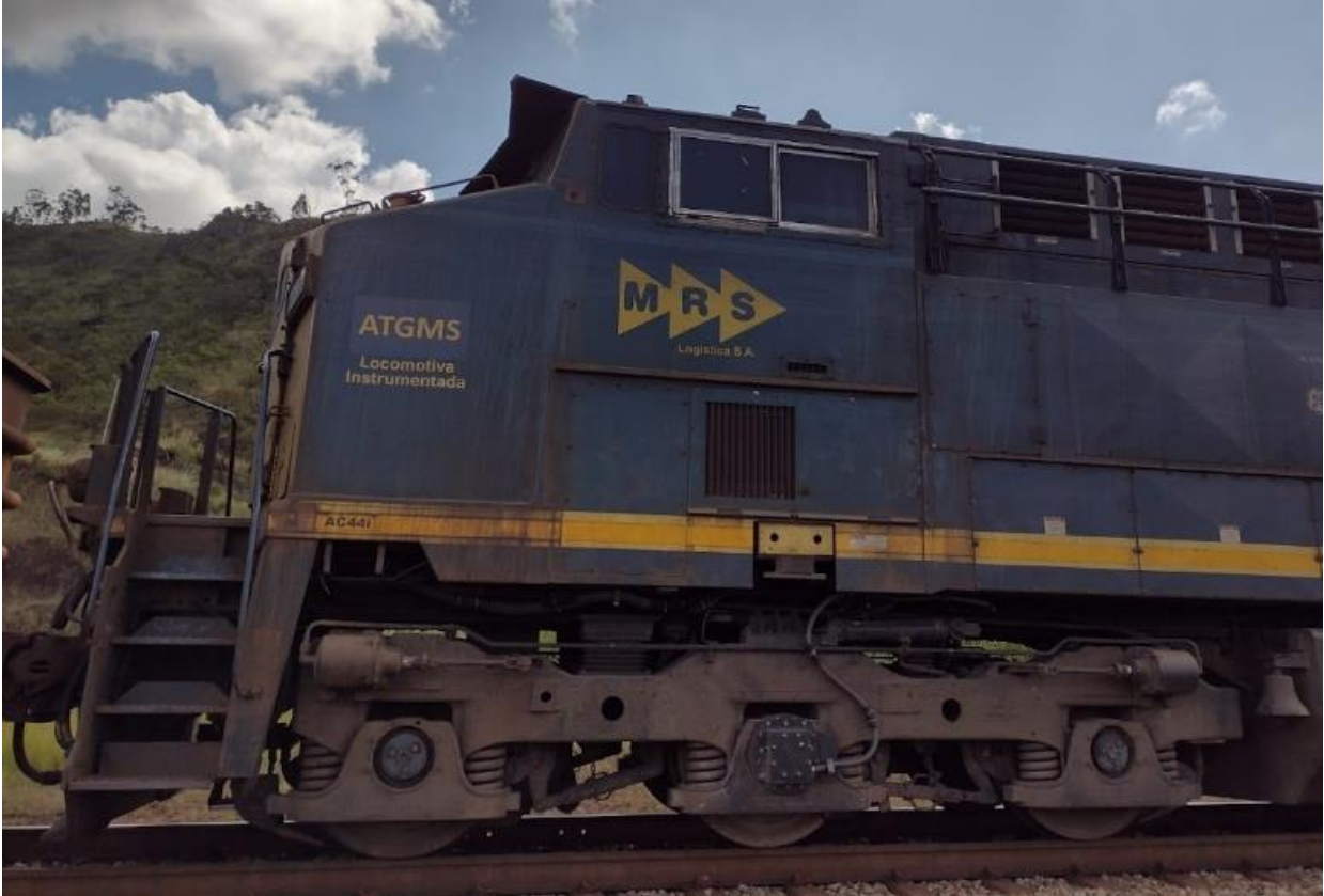
Figure 1.5: Example of locomotive mounted ATGMS used in Brazil
