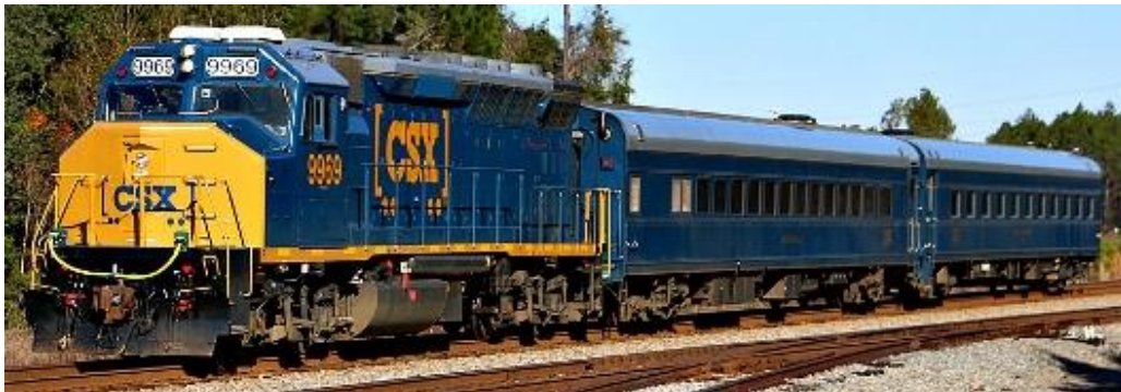
Figure 1.3: Example manned rail-bound geometry vehicle towed by a locomotive (photo credit: CSX)
