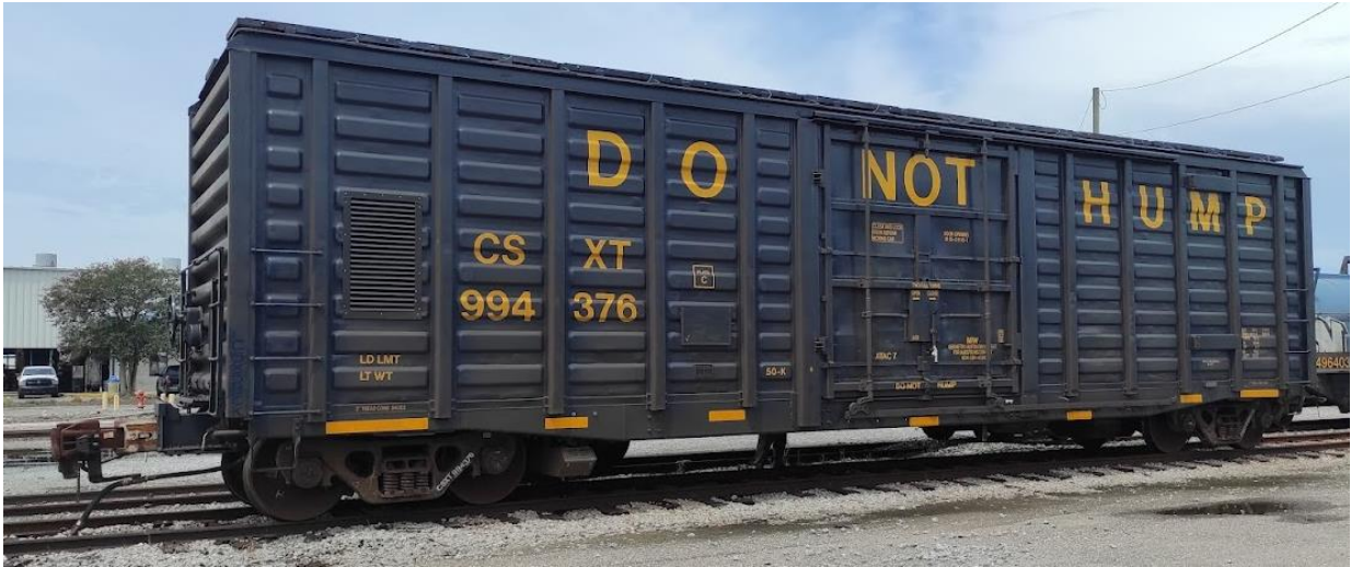
Figure 1.6: Example of boxcar mounted ATGMS used in the US
