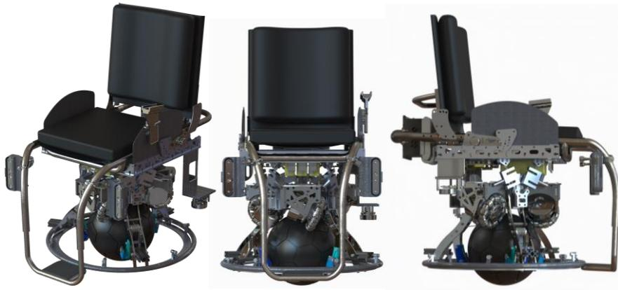
Fig. 3.1. The assistive rideable ballbot system, PURE
