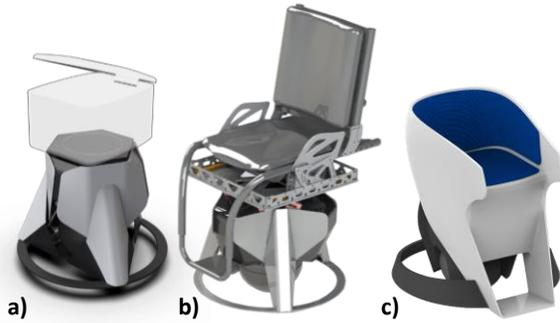
Fig. 1.2. a) PURE in payload carrying mode, b) PURE Gen2 prototype in human riding mode, and c) a concept drawing for a future generation PURE in human riding
