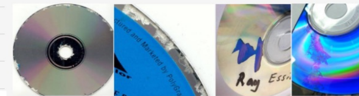
Examples of disc rot on the recording and reading surfaces of a disc [4]
