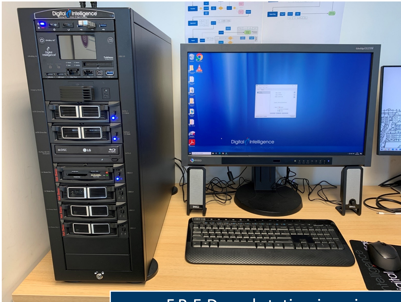
F.R.E.D workstation imaging a corrupt hard drive
