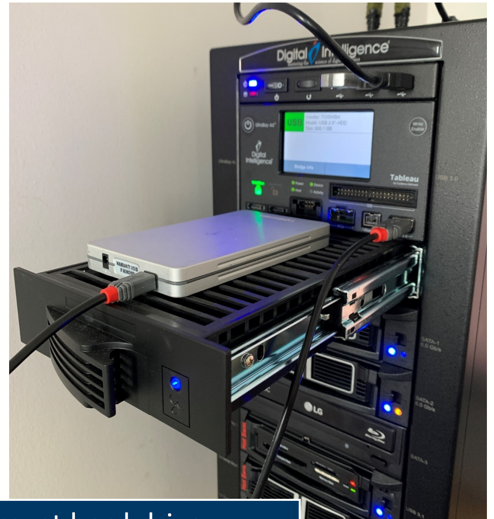
F.R.E.D workstation imaging a corrupt hard drive
