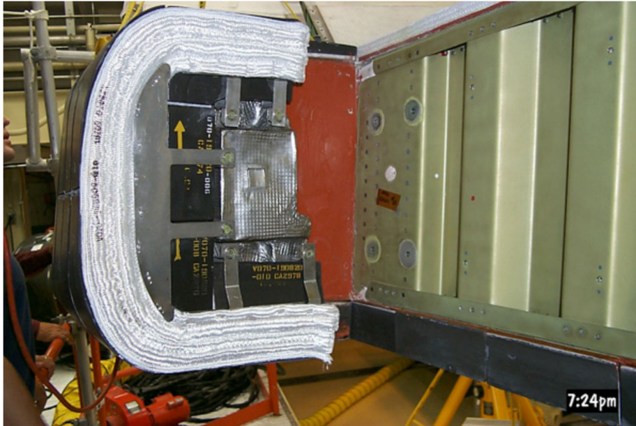
Figure 2.1: An example of a flexible thermal barrier used to seal between an RCC panel and the wingtip. The thermal barriers on the Orbiter were rated to 1093 °C. The use of aerogels in such forms of conformal insulation would afford lower thermal conductivities and lower gas permeabilities, permitting operation in more extreme environments. Image courtesy of NASA.
