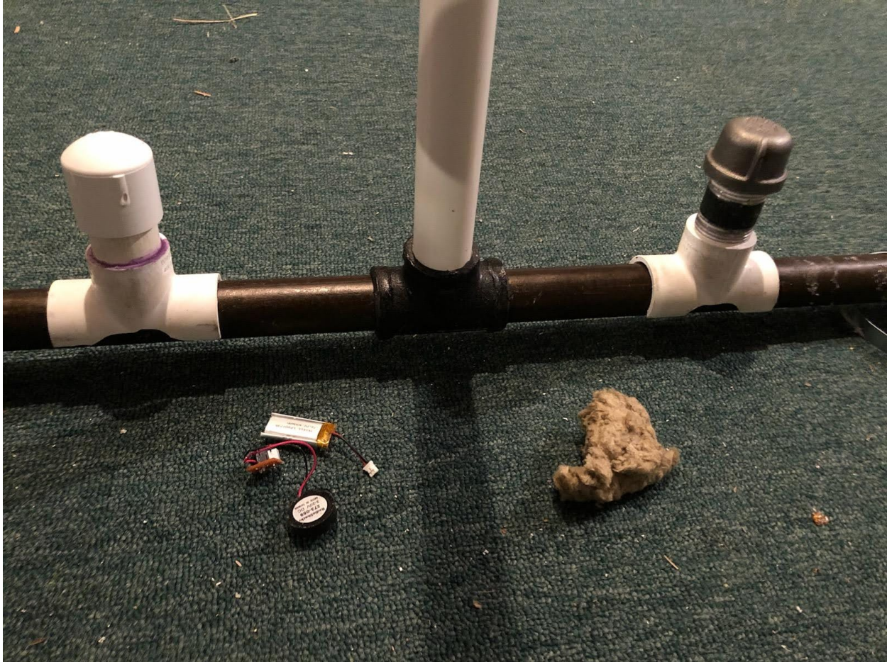
Figure 4.4: Snap Fitting Installed on Black Steel Pipe with Receiver and Rockwool
