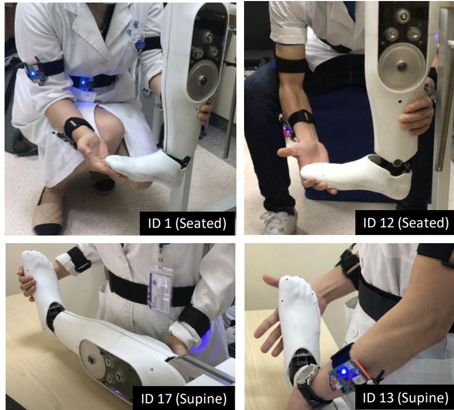
Fig. 2.4: Four subjects interacting with the simulator in two testing configurations that represented a patient in a seated or supine position [58].
