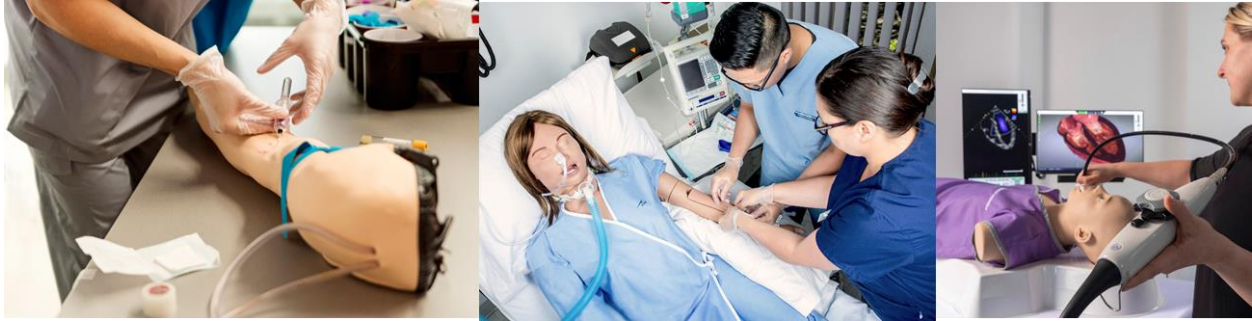
Fig. 1.2: Various commercially available medical task trainers for surgical and anatomical tasks. (A) A standalone mannequin arm for insertion procedure training [38]. (B) A full-body mannequin for nursing scenario training [39]. (C) Emergency care patient simulator for ultrasound imaging, for echocardiography training [40].
