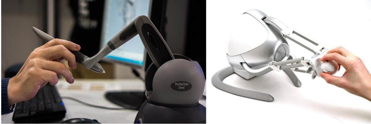
Fig. 1.3: Commercial haptic devices used together with task trainers to kinesthetic haptic feedback. (Left) Phantom Omni from 3D System [45]. (Right) Novint Falcon from Novint Technology, Inc [46].
