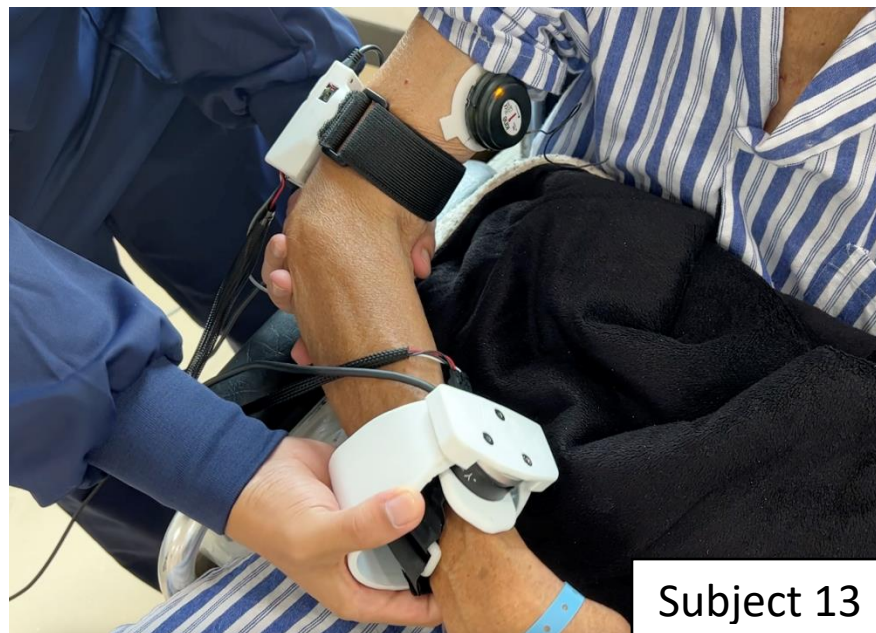
Fig. 5.7: An example photo from Subject 13 where there existed some misalignment for the upper arm IMU module as well as non-negligible shoulder abduction angle.
