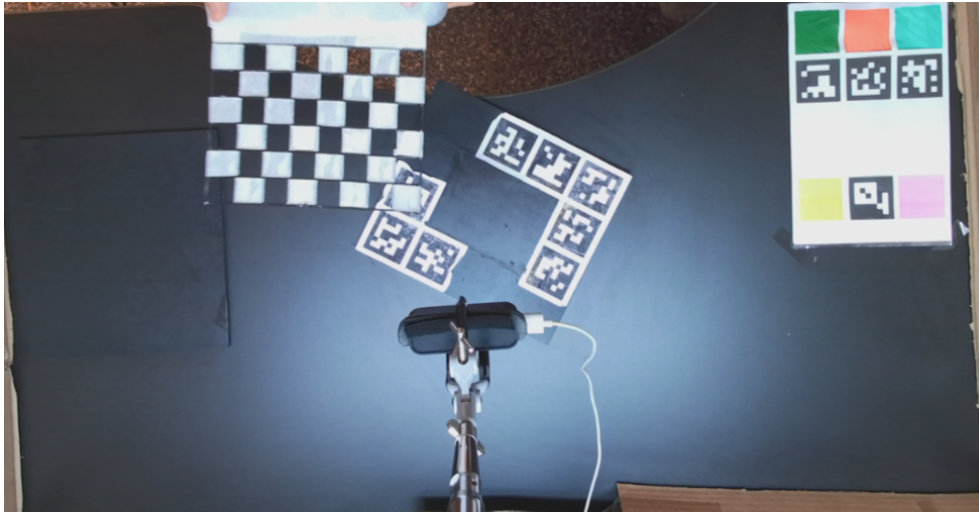
Figure 7.2: Hollow checkerboard for calibrating the depth camera of Azure Kinect DK
