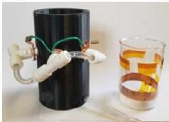
FIG. 61: 3D Printed volume for testing multiple nozzles to treat MB solution.
