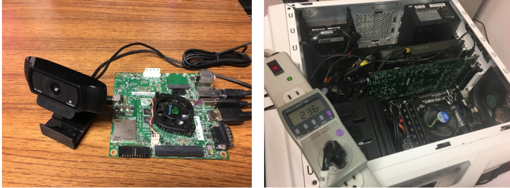
Figure 3.4: The proposed video analysis system includes a front-end (a Tegra TK1 and a webcam) and a back-end (a host PC and a Xilinx VC709 board) for performing real-time video content descriptions.
