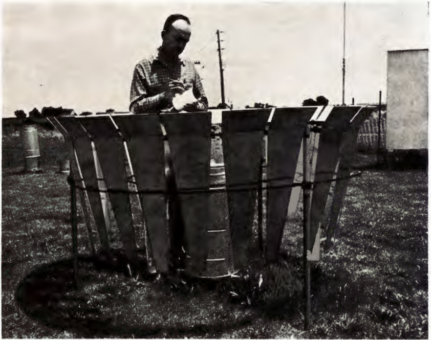
Observer reads chart from recording raingauge, which is protected by metal wind shield
