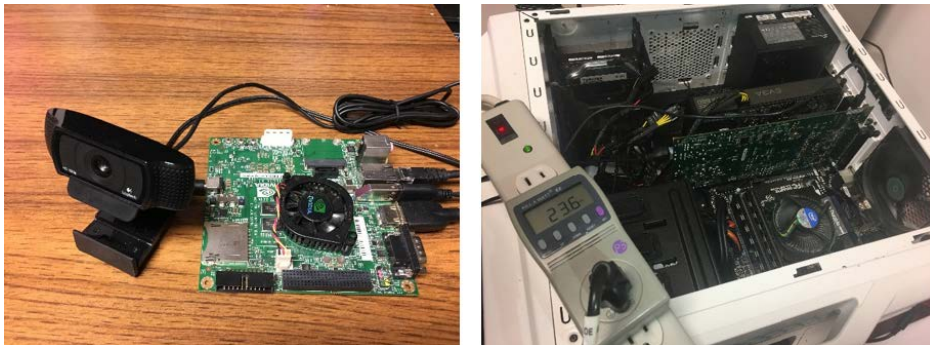
Figure 3.4: Left: Front-end (Tegra TK1 and webcam); Right: Back-end (Xilinx VC709 FPGA board, host PC)
