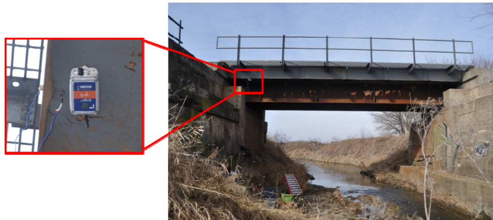
Figure 3.11 Field application of the Demand-based WSS .
