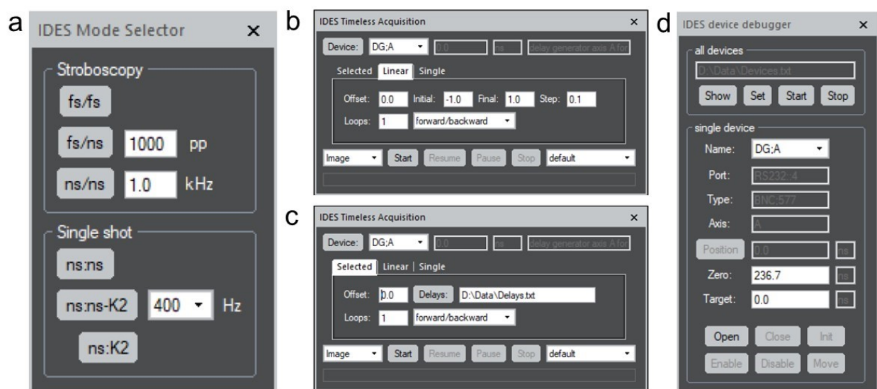
Figure 2.9: The IDES data acquisition software components in Gatan’s Digital Micrograph ® software suite. a) IDES Mode Selector interface where the user first selects the experimental modality, such as a fs pump/fs probe or fs pump/ns probe experiment. b-c) IDES Timeless Acquisition interface for the user to select the experimental parameters and start data acquisition. d) IDES Device Debugger interface for the user to monitor and debug any issue with the device controlling the temporal delay between pump and probe.
