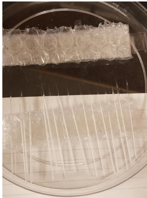
Figure F.4: Micropipettes of OD of 1 mm and ID 0.58 mm and the tip being \sim 3 \mu\text{m} for aspirating red blood cells and MSCs after microforging.
