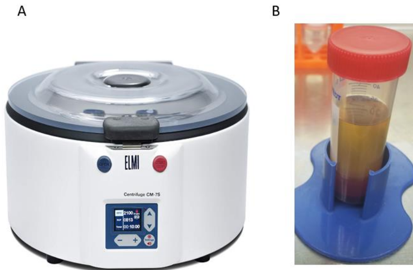
Figure F.9: (A) Benchtop centrifuge for isolating red blood cells from whole blood and (B) Red blood cells isolated (bottom) from whole blood (top) after centrifuging for 20 mins at 1200 g (rcf).
