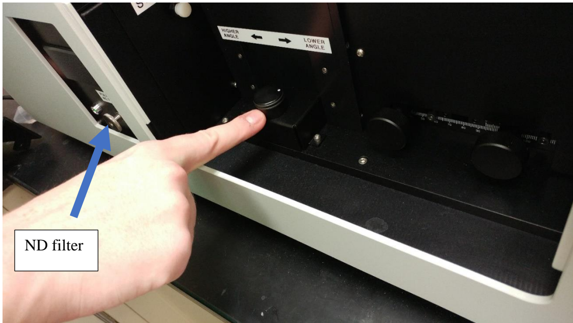
Figure E.7: The location of the ND filter and the knob that controls the incident angle of light
