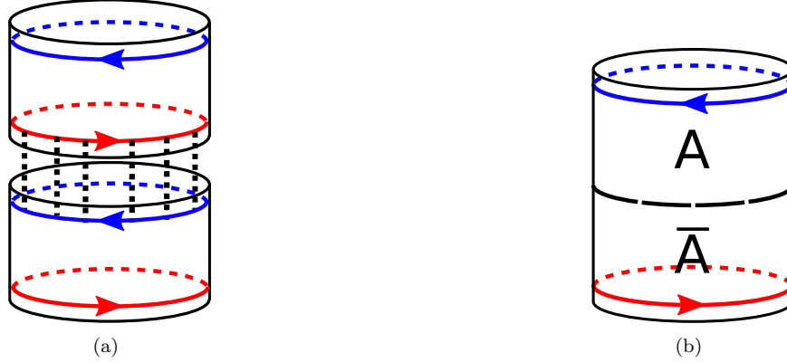
Figure 1.1: (a) Cartoon of a gapped interface. The two cylinders support (possibly distinct) topological orders. The red and blue arrows denote the chiral edge states. The dotted lines between the inner edges represent electron scattering terms, which gap out the interface. (b) Spatial bipartition involved in computation of the entanglement entropy.
