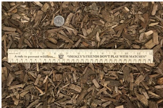
Figure 73. Large-scale photograph of Chip #15 depicting visual size distribution. Ruler top and bottom gradations in inches and centimeters, respectively.
