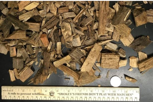
Figure 85. Large-scale photograph of Chip #18 depicting visual size distribution. Ruler top and bottom gradations in inches and centimeters, respectively.
