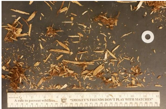
Figure 45. Large-scale photograph of Chip #8 depicting visual size distribution. Ruler top and bottom gradations in inches and centimeters, respectively.
