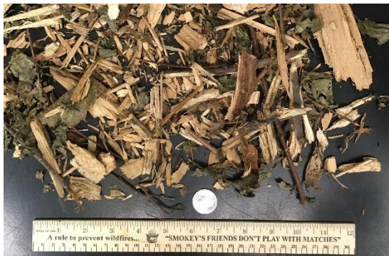
Figure 53. Large-scale photograph of Chip #10 depicting visual size distribution. Ruler top and bottom gradations in inches and centimeters, respectively.
