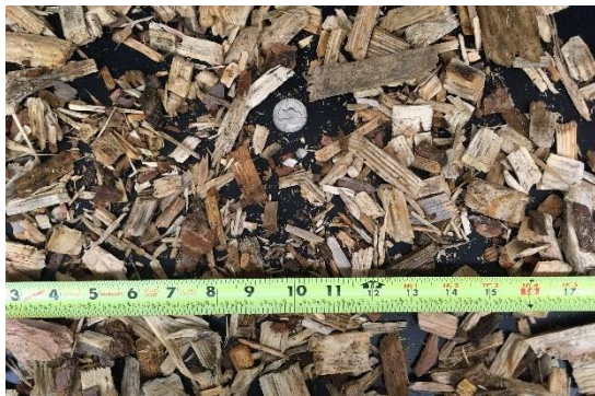
Figure 89. Large-scale photograph of Chip #19 depicting visual size distribution. Ruler top and bottom gradations in inches and centimeters, respectively.
