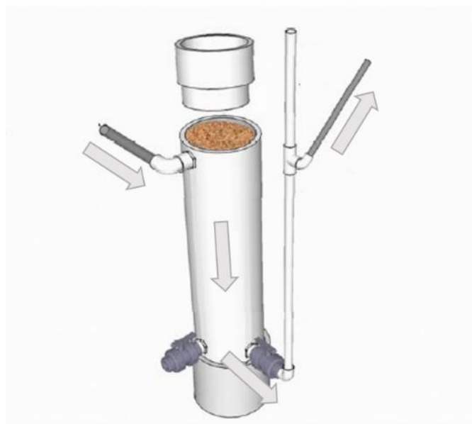
Figure 6. “Chipometer” Permeameter constructed in the ABE Hydraulics Lab at the University of Illinois.
