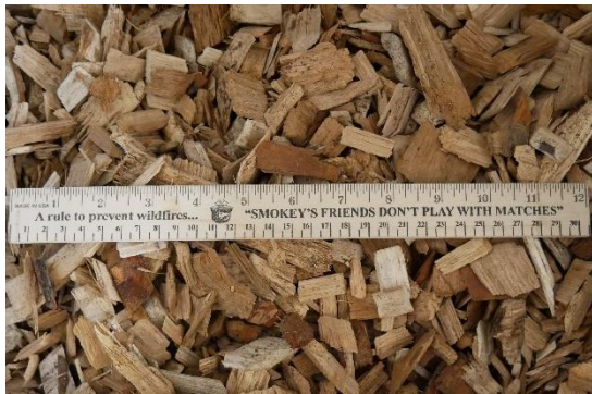
Figure 65. Large-scale photograph of Chip #13 depicting visual size distribution. Ruler top and bottom gradations in inches and centimeters, respectively.
