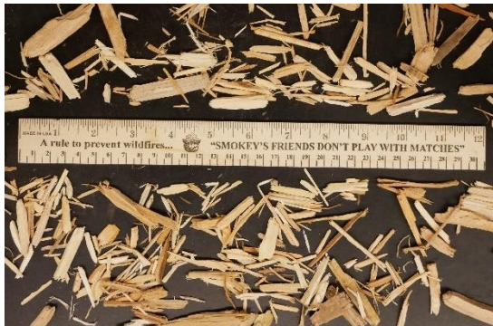
Figure 33. Large-scale photograph of Chip #5 depicting visual size distribution. Ruler top and bottom gradations in inches and centimeters, respectively.
