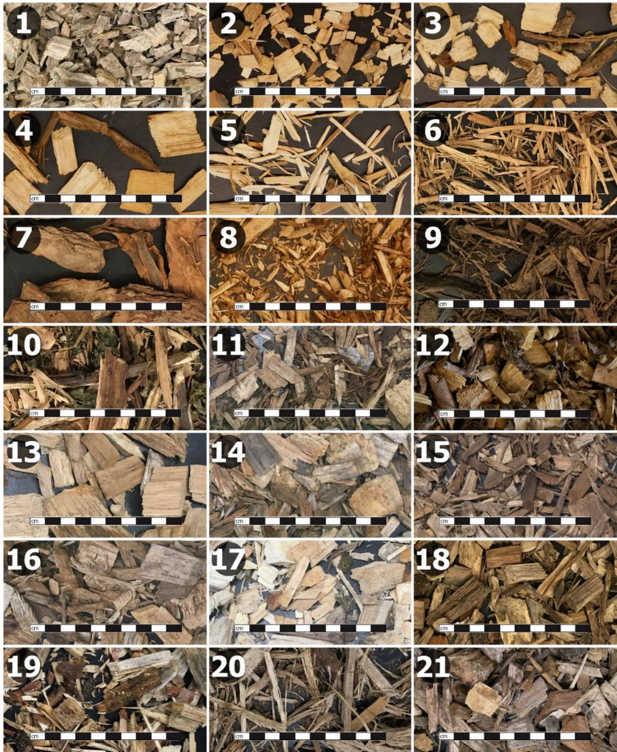
Figure 1. Photo illustration of twenty-one woodchip types commonly available in the Midwest (IL, IA, MI) evaluated for physical and hydraulic properties.
