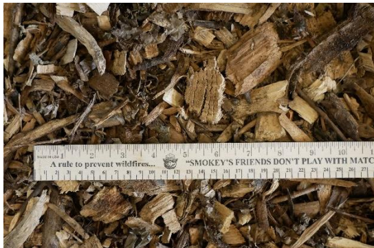
Figure 61. Large-scale photograph of Chip #12 depicting visual size distribution. Ruler top and bottom gradations in inches and centimeters, respectively.
