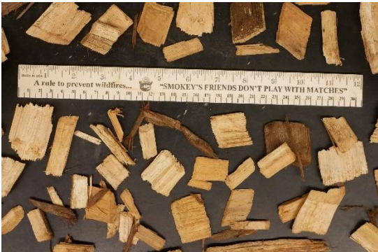
Figure 29. Large-scale photograph of Chip #4 depicting visual size distribution. Ruler top and bottom gradations in inches and centimeters, respectively.
