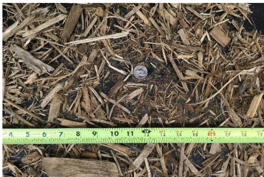
Figure 93. Large-scale photograph of Chip #20 depicting visual size distribution. Ruler top and bottom gradations in inches and centimeters, respectively.
