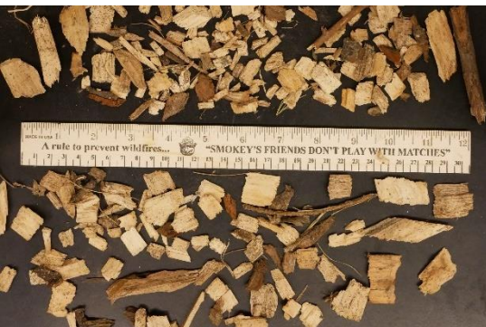
Figure 25. Large-scale photograph of Chip #3 depicting visual size distribution. Ruler top and bottom gradations in inches and centimeters, respectively.
