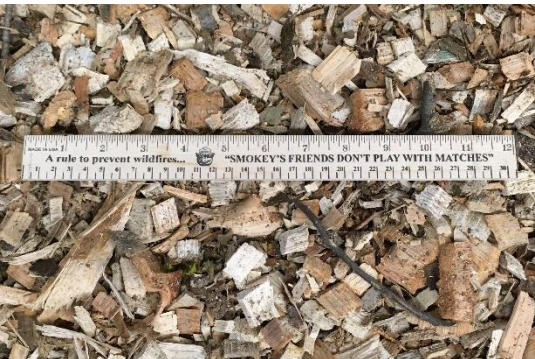
Figure 81. Large-scale photograph of Chip #17 depicting visual size distribution. Ruler top and bottom gradations in inches and centimeters, respectively.
