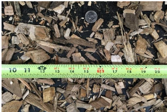
Figure 97. Large-scale photograph of Chip #21 depicting visual size distribution. Ruler top and bottom gradations in inches and centimeters, respectively.
