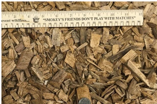
Figure 77. Large-scale photograph of Chip #16 depicting visual size distribution. Ruler top and bottom gradations in inches and centimeters, respectively.
