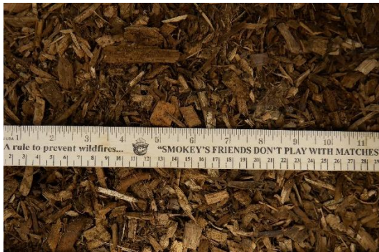
Figure 57. Large-scale photograph of Chip #11 depicting visual size distribution. Ruler top and bottom gradations in inches and centimeters, respectively.
