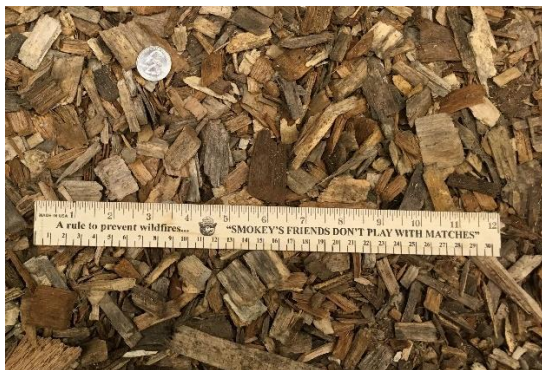
Figure 69. Large-scale photograph of Chip #14 depicting visual size distribution. Ruler top and bottom gradations in inches and centimeters, respectively.
