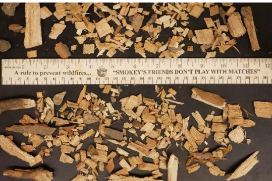
Figure 21. Large-scale photograph of Chip #2 depicting visual size distribution. Ruler top and bottom gradations in inches and centimeters, respectively.
