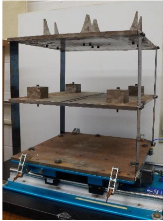
Figure 3.11 Two-story structure onboard a shake table
