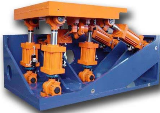
Figure 1.4 Load and Boundary Condition Box (LBCB)
