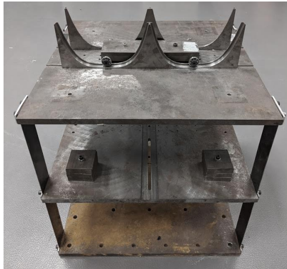
Figure 4.3 Two-story steel frame with track NES
