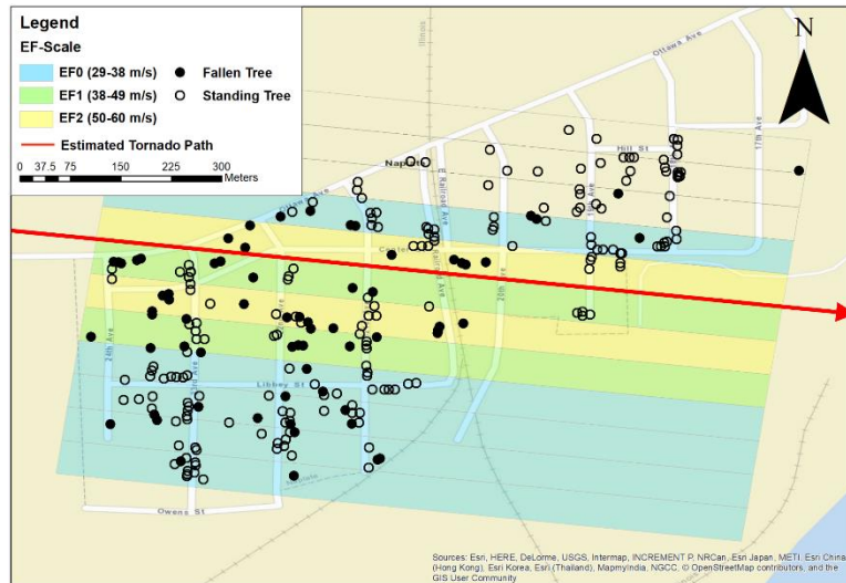
Figure 7.2. Documentation of fallen trees and standing trees and near-surface wind field estimation of Naplate, IL using the “modified” Godfrey-Peterson method.
