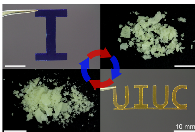
Figure 2.8. Photographs of solvent cast cPPA films (dyed with methylene blue or Astrazon Orange R during the casting process and laser cut into specified shapes for visualization) and the monomer ( o PA) collected following depolymerization of the dyed films. The dyed films are held by metal tweezers. Blue arrows represent polymerization and film casting, and red arrows represent depolymerization and monomer collection.
