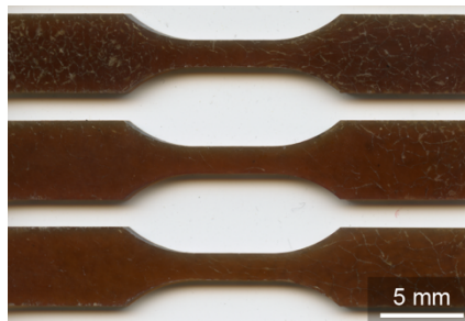
Figure 2.13. Optical images of cPPA dogbones (2.5 phr DPP, 0.5 phr DBPDA) pressed at 20 MPa and 110 °C for 15 minutes.
