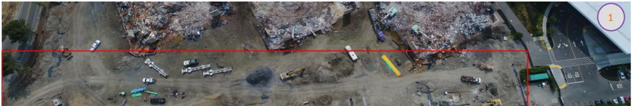
Figure 3.2: Site-camera configuration for the voyager dataset. The red bounding box marks the area monitored, the circle on the top right corner marks the position of the camera mounted on a tripod. The monitored area is 270 meters in width and 35 meters in height.
