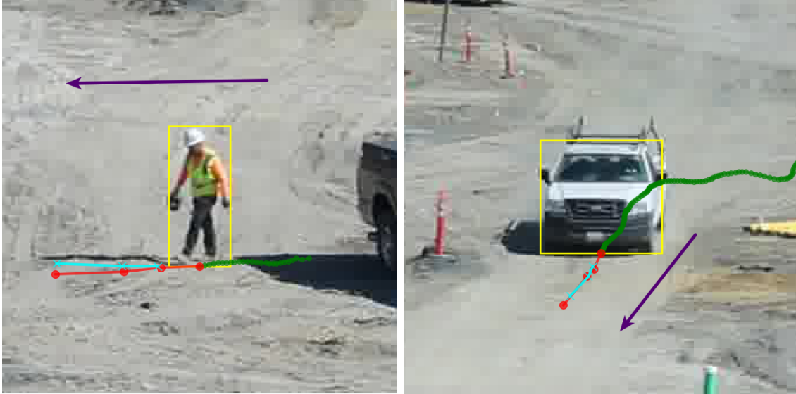
Figure 3.6: Examples of path prediction generated from the final model. Tracks of the lower center of bounding boxes are treated as the object track. The green track represents previously observed locations; the red dot line represents the current location and the actual future locations; the cyan cross line represents the model predictions. The arrows indicate the forward moving directions. Figure best viewed in color.
