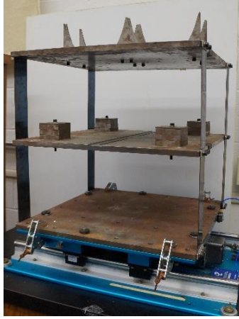
Figure 3.11 Two-story structure onboard a shake table
