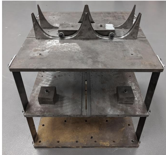
Figure 4.3 Two-story steel frame with track NES
