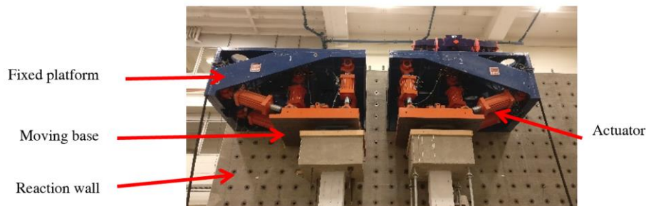
Figure 2.14 Load and Boundary Condition Boxes at the University of Illinois at Urbana-Champaign
