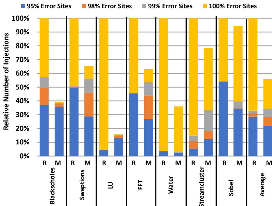
Figure 3.3: Number of error injections for different error-site coverage targets for each benchmark, relative to 100% error-site coverage for Ref (Ref100). R=Ref, M=Min.
