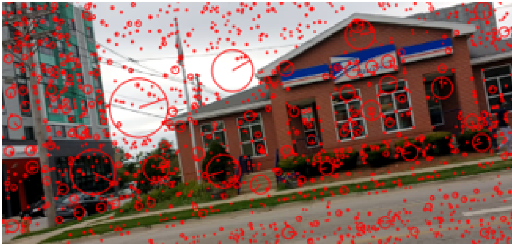
Figure 1.3: SIFT features are shown as red circles with a direction. The urban environment is abundant with unique features which improve localization using a vision-based approach.
