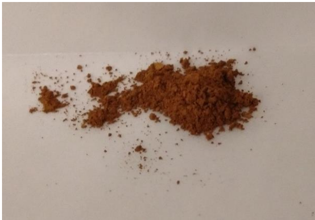
Figure 26. The color of the crystallized GTDHEO powder sample. Based on the yellowish-brown color, trivalent and tetravalent terbium might have coexisted in the bixbyite structure.
