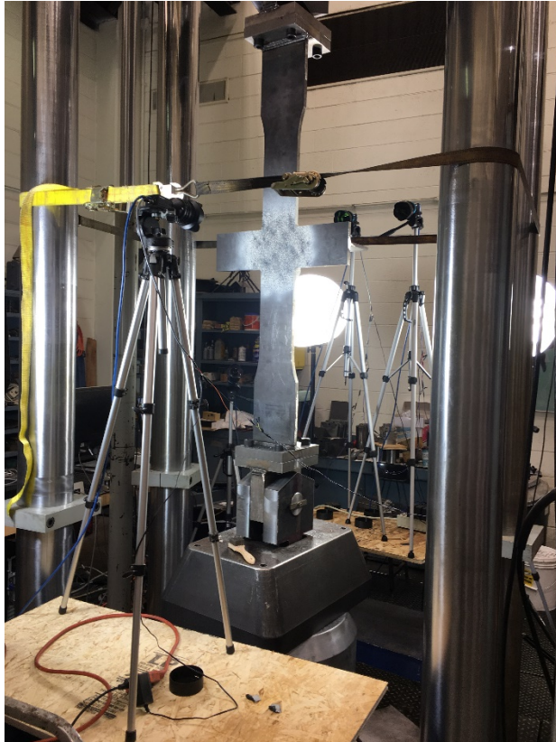
Figure 7.3. Specimen of typical miter gate welded cruciform joint in load frame for fatigue testing.
