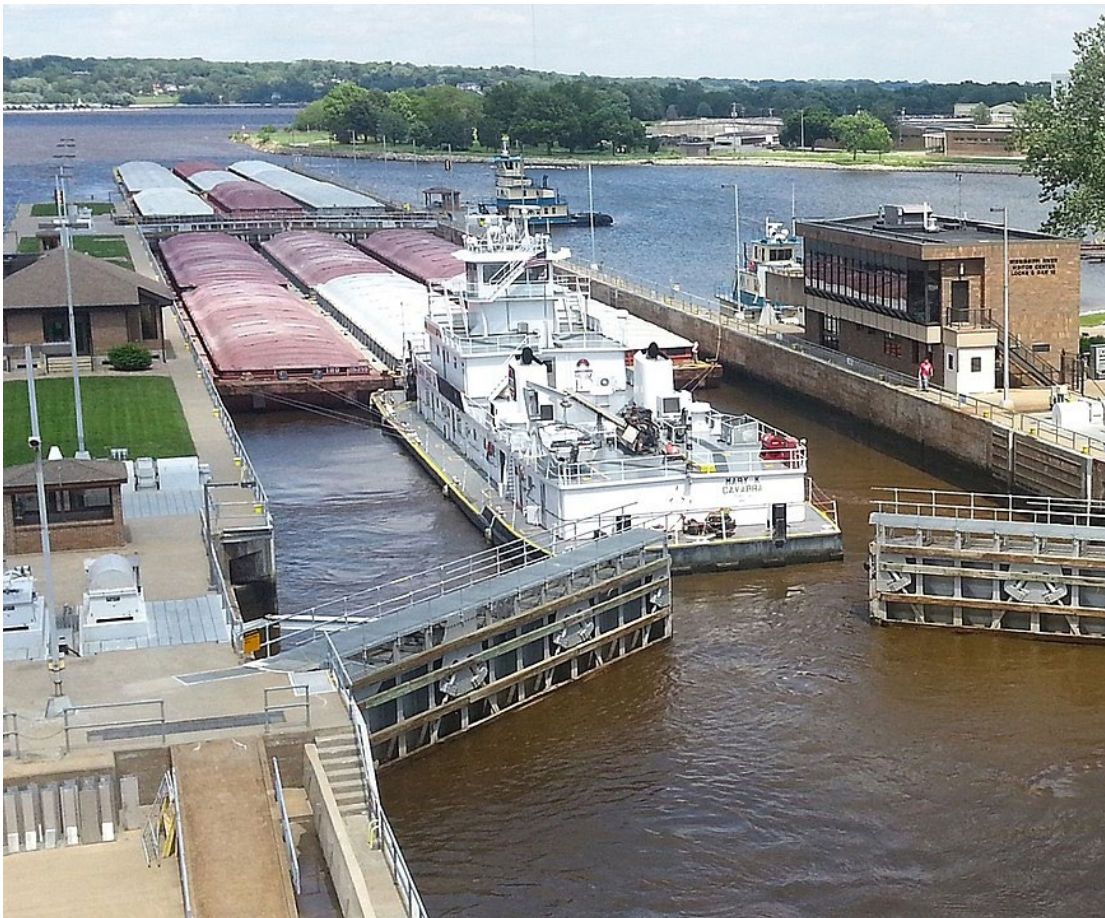
Figure 1.2. Typical towboat carrying 15 barges through a lock site (U.S. Army Corps of Engineers n.d.).
