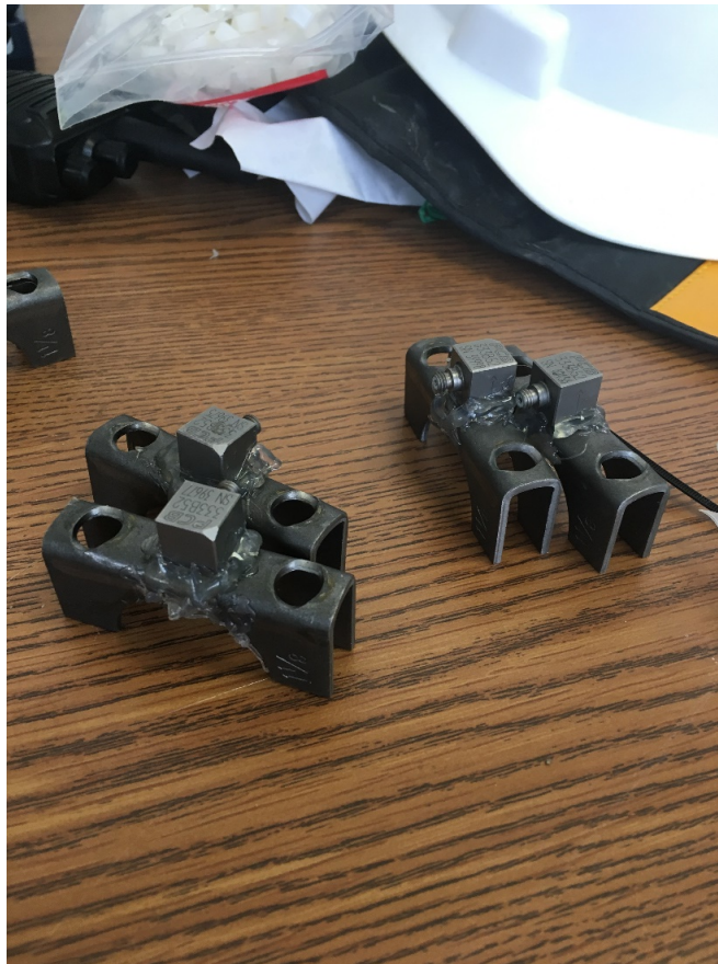
Figure 6.7 Accelerometers attached to the U-bracket.
