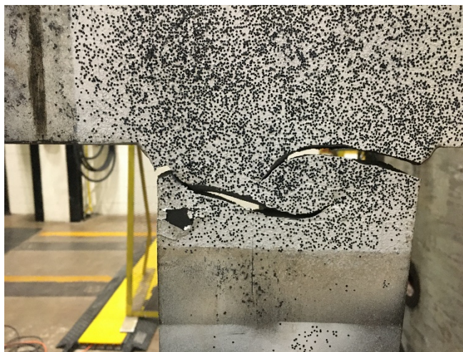
Figure 7.4. Successful formation and propagation of cracks (note speckle patterns for DIC).
