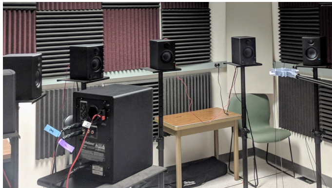
Figure 2.5: Studio monitors are used to simulate human talkers.
