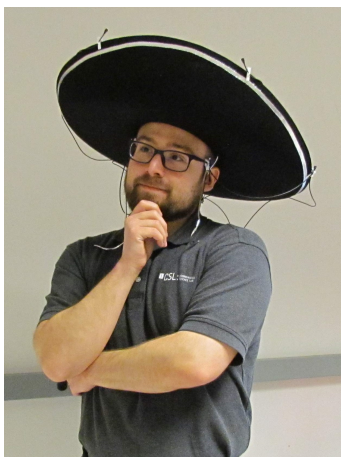
Figure 1.6: Large wearable microphone arrays such as the Sombreato can provide better spatial resolution than microphones worn on the ears.
