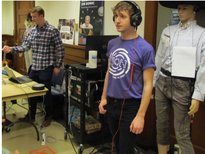
Figure 2.4: A mobile recording cart houses a 16-input, 10-output digital audio interface attached to a fanless computer. It can be used for field experiments and live demonstrations.
