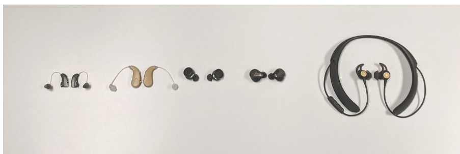
Figure 1.2: There are many kinds of listening devices on the market, including hearing aids (left), “hearables” (center), and advanced headphones (right).
