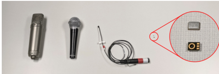
Figure 9.2: From left to right: A large-format cardioid condenser microphone, a dynamic vocal microphone, an omnidirectional lavalier microphone, and a MEMS microphone.
