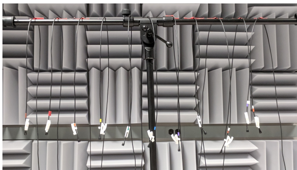
Figure 2.1: An array of omnidirectional lavalier microphones.
