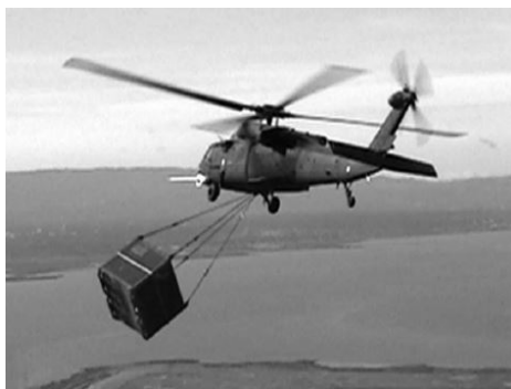
Figure 2.3: Flight test with full-scale slung loads; adapted from [52].
