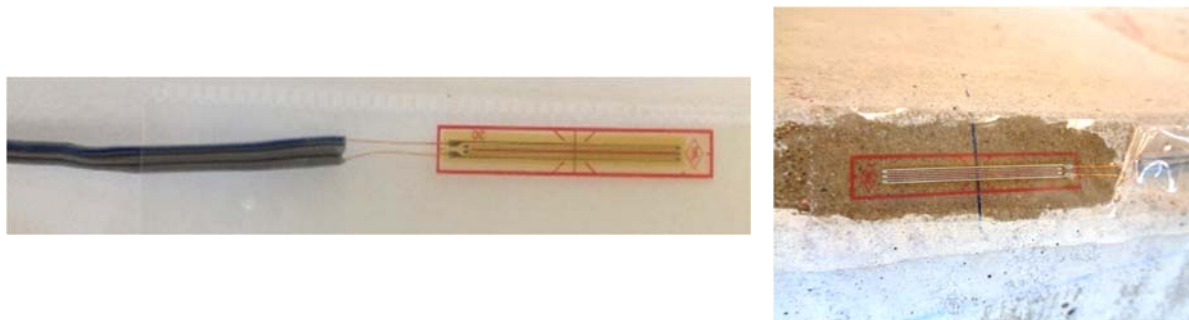
Figure 2.1: Standard 120-Ohm concrete strain gauge before (left) and after (right) installation on concrete crossie (Wolf, 2015b).
