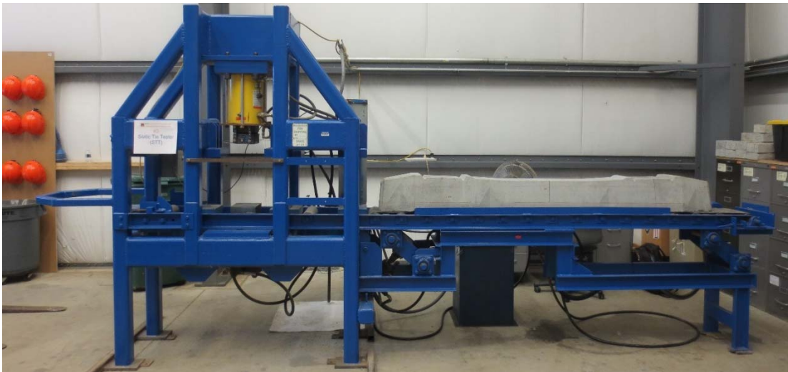
Figure 2.6: Static Tie Tester (STT) at UIUC used for laboratory calibration of concrete crossties.
