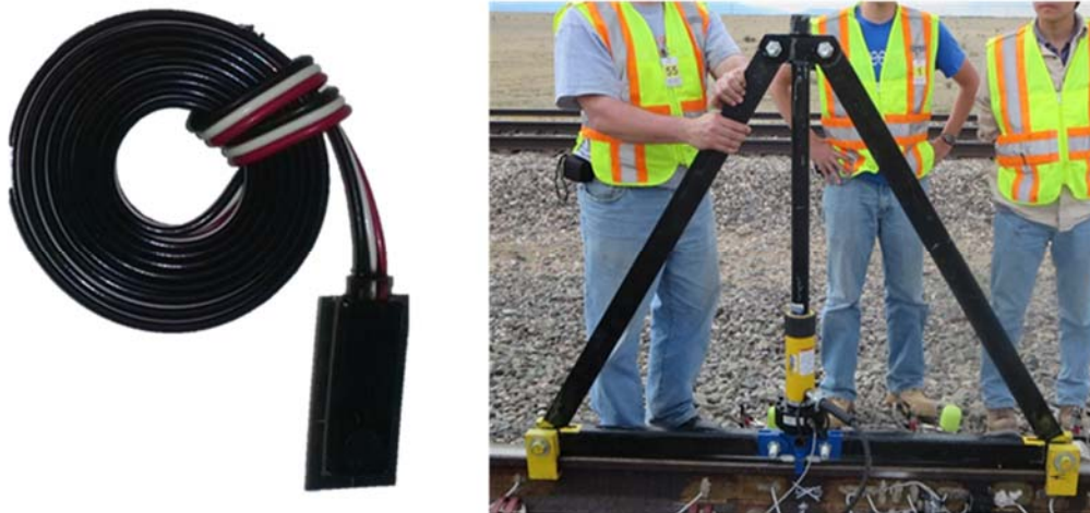
Figure 3.3: Weldable half-bridge shear strain gauge (left) and loading frame used to calibrate gauges by relating strain to known system input load (right).
