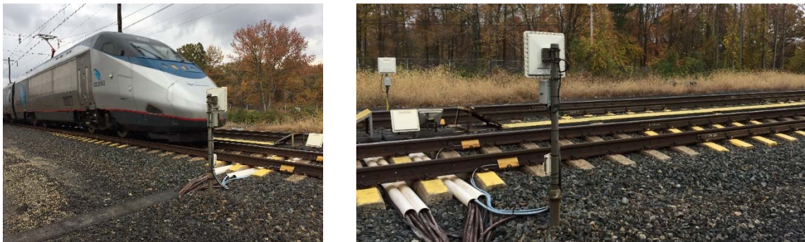
Figure 3.2: Wheel Impact Load Detector (WILD) on Amtrak’s Northeast Corridor at Edgewood, MD; used to capture the commuter rail train loads in this chapter.
