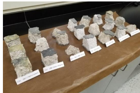
Strength cubes after UCS testing
