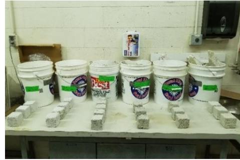
Saw-cut cubes from different sections
