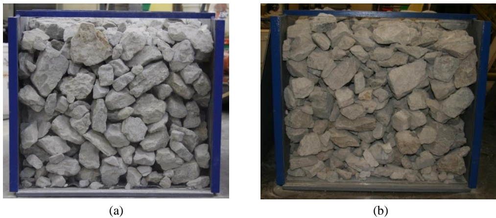
Figure A.1 Cross section of the compacted PCR aggregates in (a) one lift and (b) two lifts
