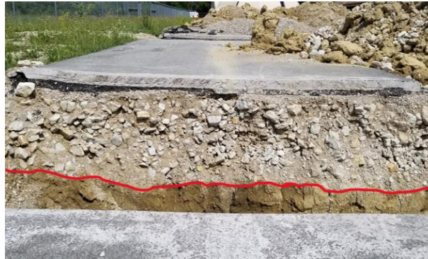
C1S2E – PCR/QB1 in 1 Lift
