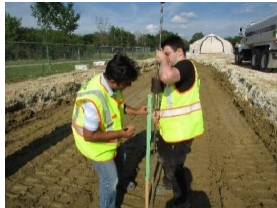
DCP profiling for top 305 mm (12 in.)
