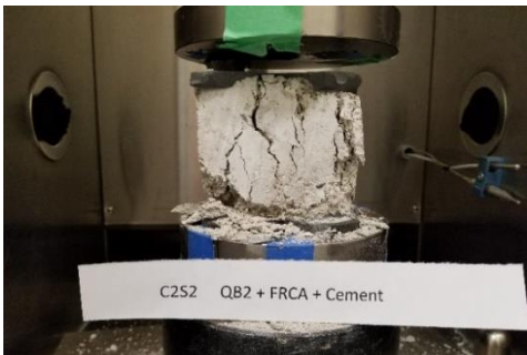
UCS testing of a cube
