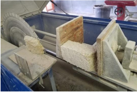
Saw-cutting cubes for strength testing
