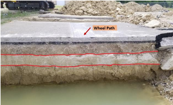
C3S2W – QB2 + Cement Subbase & CA06_R Base
