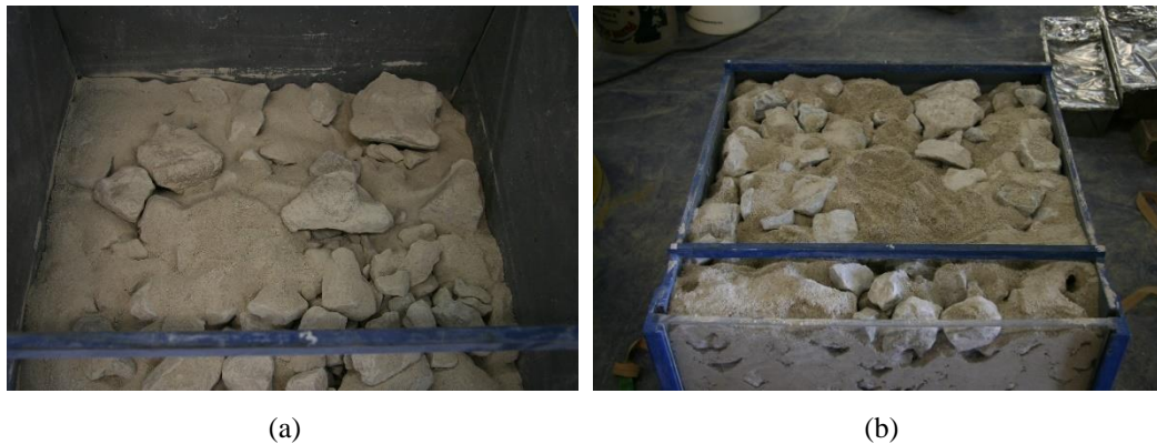
Figure A.4 Top view of the surface of the compacted PCR aggregates with (a) 40% dry QB and (b) 30% wet QB (moisture content = 2.5%), showing roughly similar quantities remaining on the surface
