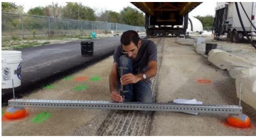
Customized rut depth measuring device
