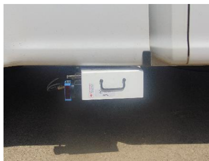
(b) Accelerometer and laser-beam source
