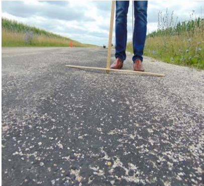
(a) Rut-depth measurement
