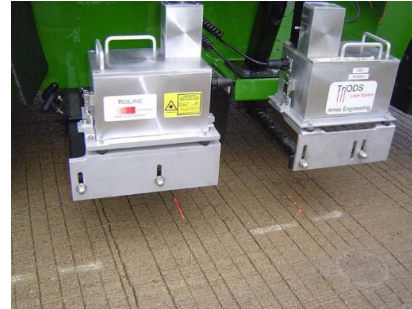
(b) Lightweight profilometer with sensors
