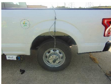
(a) High-speed profiler mounted on truck and displacement transducer attached to the wheel
