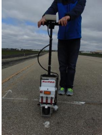
(a) A walking profilometer used by IDOT
