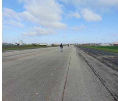
(b) Track to calibrate walking profilometer; white dots indicating driving path
