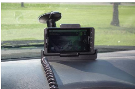
(a) A cell phone mounted on the car to measure IRI
