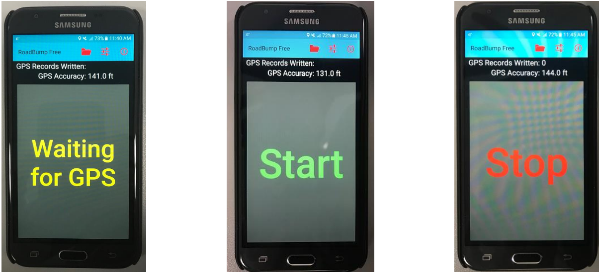
Figure C-26. GPS for site location, start and stop the data collection options to collect data.
