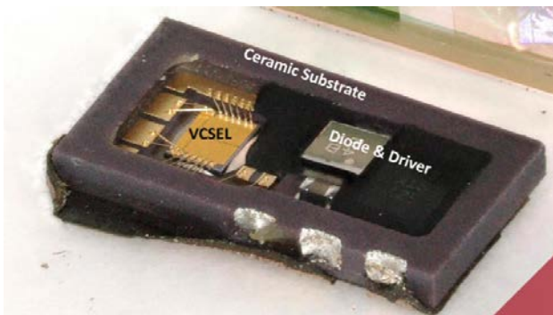
Figure 1.1 NIR dot projector in the iPhone X for Face ID. Image courtesy of Systems Plus Consulting [5]
