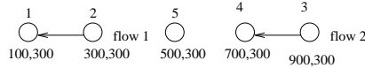
Figure 3.7: Scenario for channel estimation experiment in the presence of hidden flow effects.
