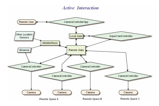
Figure 1. Interaction between the various application components and the middleware infrastructures.
