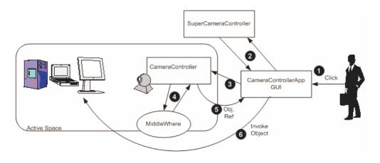
Figure 2. Control flow protocol for remote interaction. Describes the steps involved in the user interaction with a remote object.
