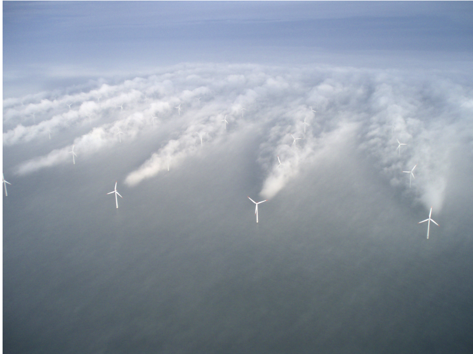
Figure 1.2: Wind-turbine wakes are visualized by fog formation in the Horns Rev 1 wind farm. Photo by Christian Steiness.
