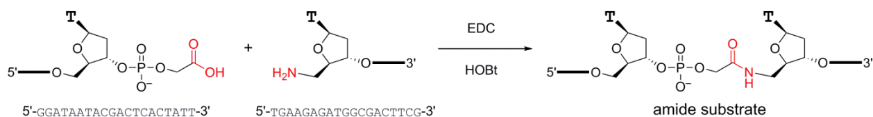
Figure 2.21. Synthesis of amide substrate by splinted coupling of 3'-CO 2 H oligonucleotide and 5'-amino-5'-deoxythymidine oligonucleotide.
