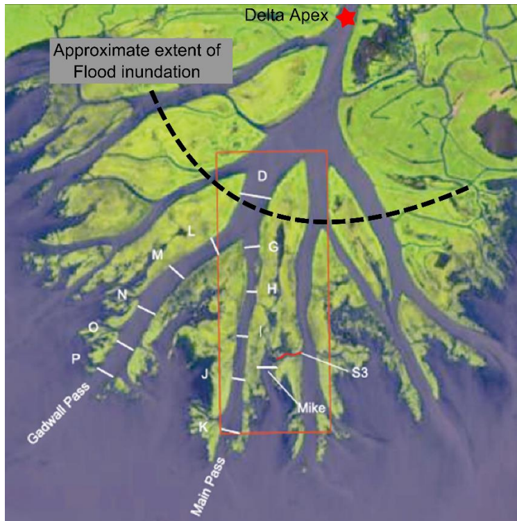
Figure B-1: Figure modified from Hiatt and Passalacqua (2015). An approximation of the typical flooding length scale r_{flood} from results of Gelensye et al (2015) can be estimated from the distance to the shoreline during floods. The lettered cross sections represent locations where discharge was measured in Gadwall Pass and Main Pass.
