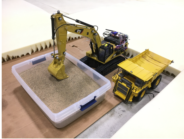
Figure 1.1: An excavator robot and its human operator performing a truck loading task in a safety critical and dynamically changing environment. Our goal is to enable construction robots to learn instructional policy from skilled human operators, and use that policy to guide and train novice human operators in completing complex tasks.
