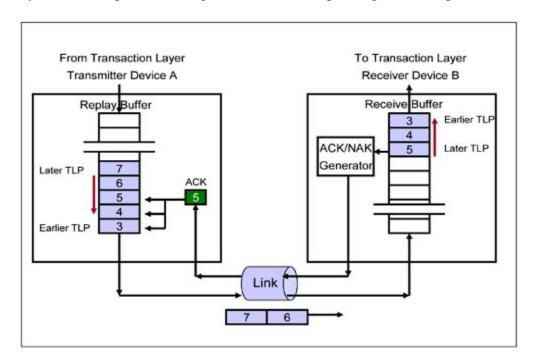
Fig. 3.9 Ack/NAK protocol example in a real system [17]
