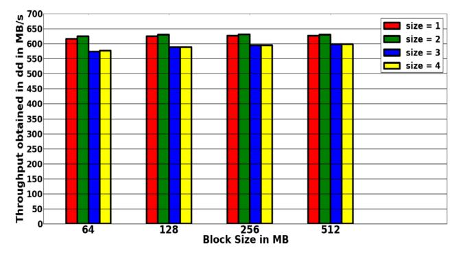
**5.3** Comparing the Performance of the IDE Disk Using x8 Links, Different Replay Buffer Sizes
