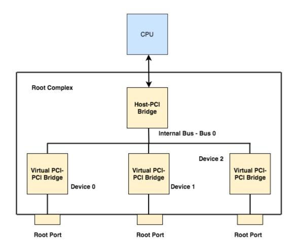
Fig. 3.4 Internal structure of root complex in a real system
