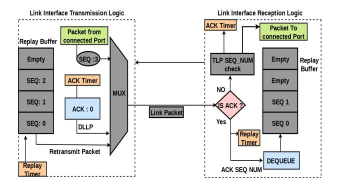
Fig. 3.10 Link interface transmission and reception logic
