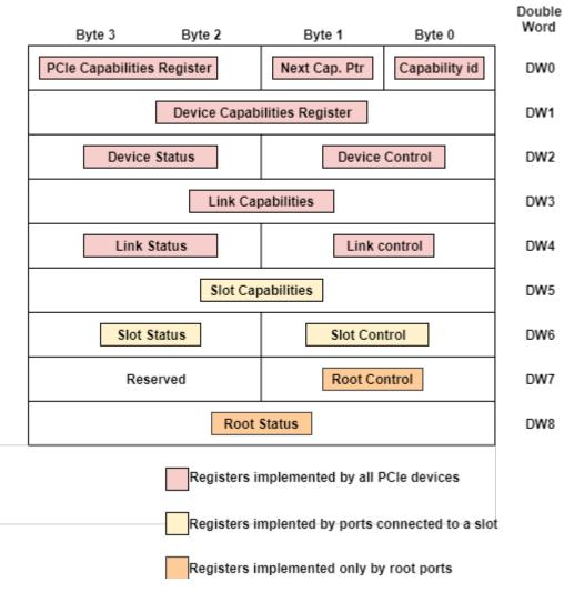
Fig. 3.2 PCI Express capability structure
