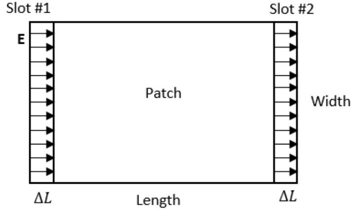
Figure 5. Top view of the cavity model adapted from [10].
