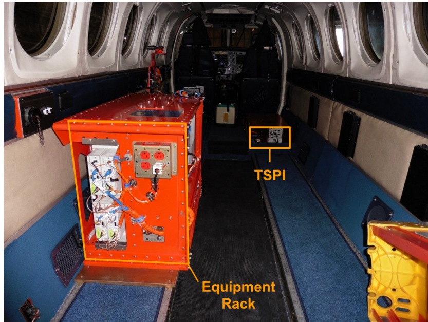
Figure 4.3: Equipment rack (bright orange) as installed on board the flight test aircraft. Four USRPs are immediately visible in the bottom-left corner. CSAC is hidden from plain view. The TSPI system (white, orange) is mounted on the floor directly behind the co-pilot’s seat.
