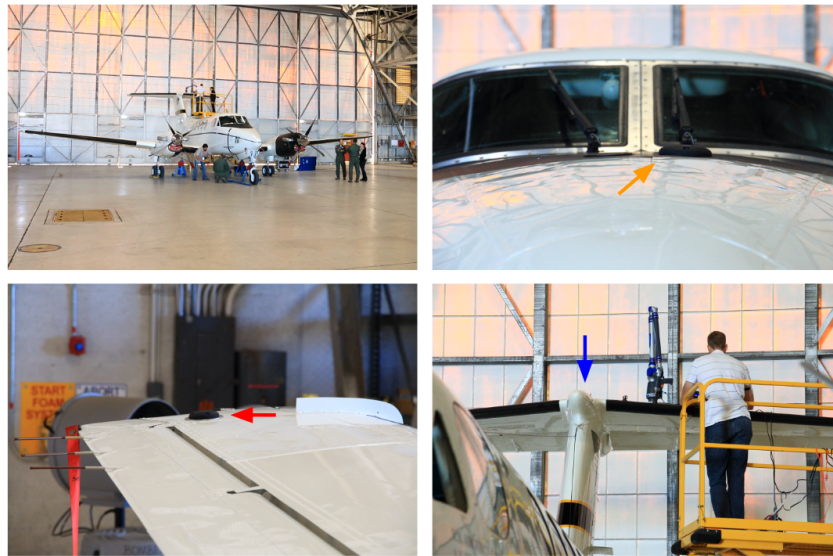
Figure 4.2: Clockwise from top left: flight test aircraft, C-12C Huron; nose antenna (in front of cockpit canopy); tail antenna (on top of vertical stabilizer, not visible) and the measuring of antenna baselines using FARO ® FaroArm portable coordinate measuring machine (PCMM); left-wing antenna.
