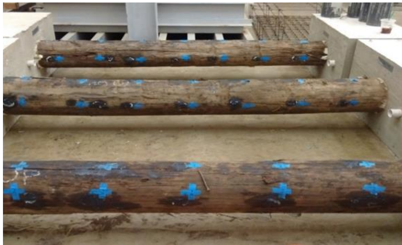
Figure 4.1 Timber pile specimens used in experimental testing of FRP retrofits
