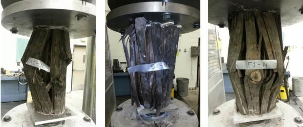
Figure 3.5 Failure of unretrofitted timber specimens
