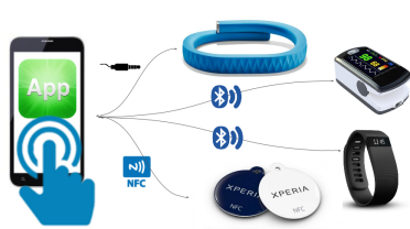
(a) Smartphone apps compete for connectivity resources to access personal IoT devices.
