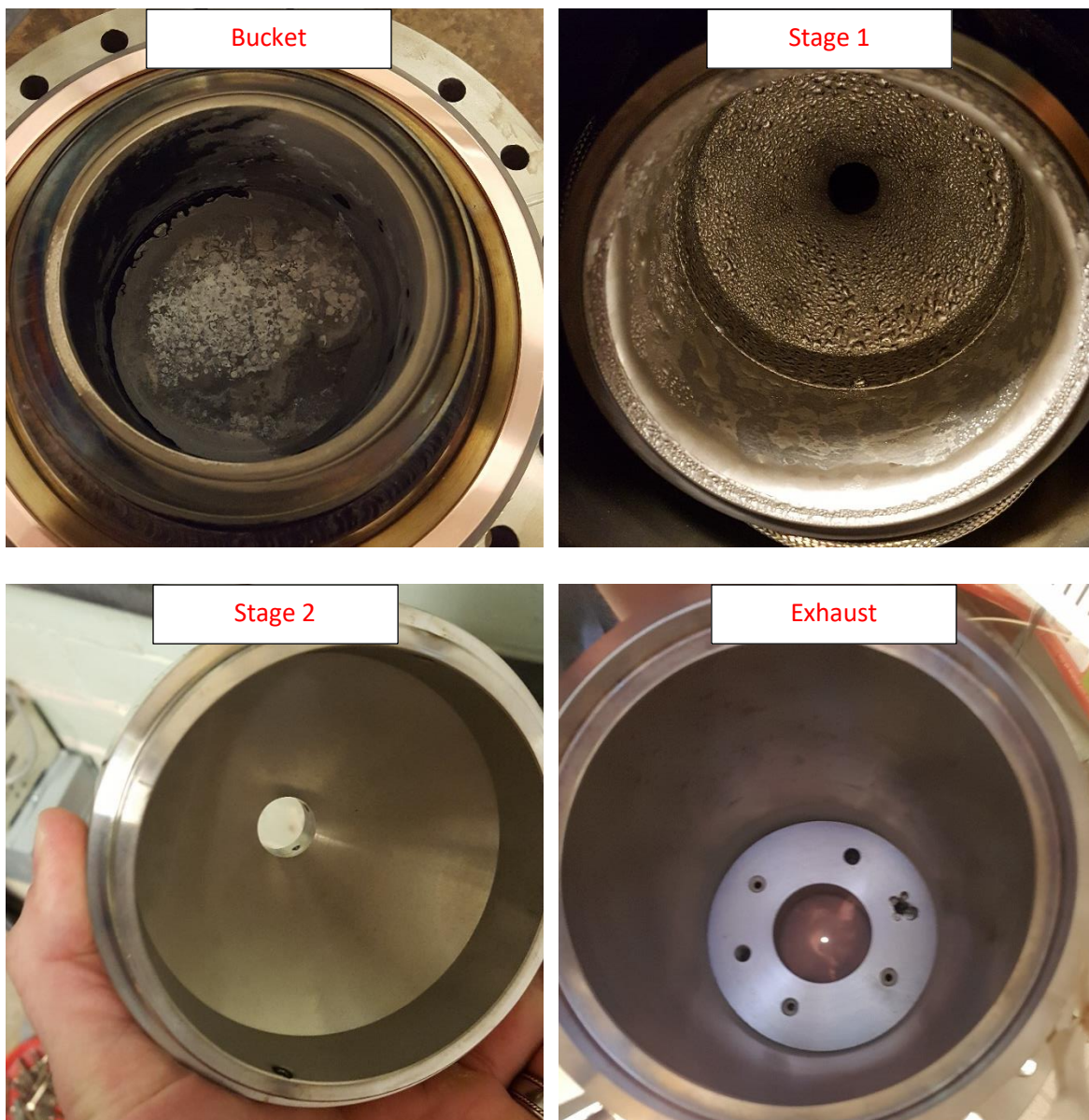
Figure 6.15: Images of the internal components of the column post mortem. The majority of the Li condenses on the bottom of Stage 1; however, some Li residue was noticeable on Stage 2 and the Exhaust.
